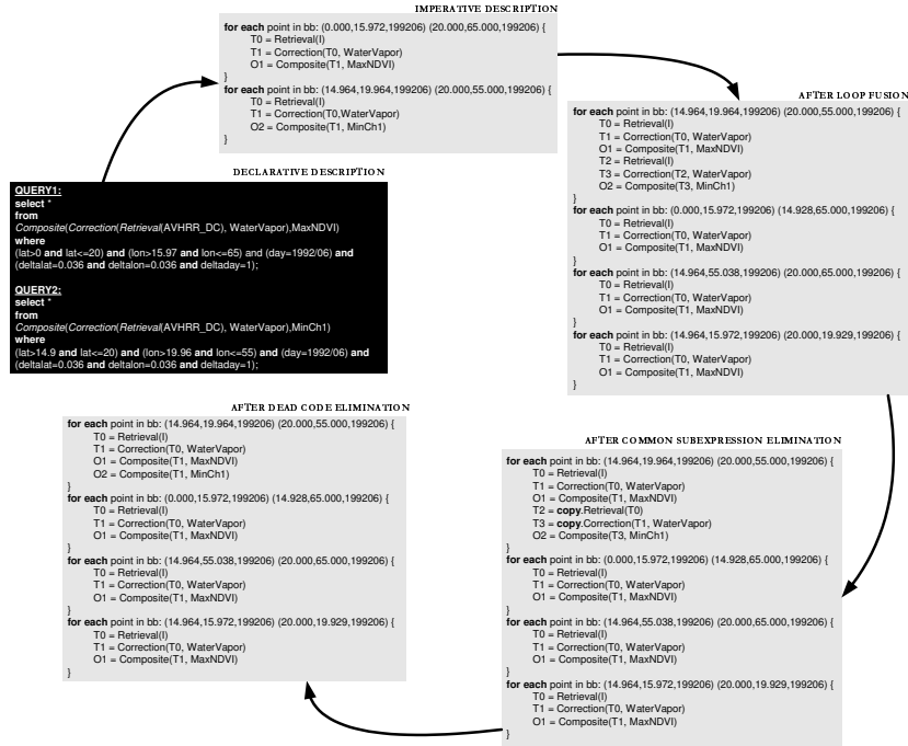
Fig. 2. An overview of the entire optimization process for two queries. MaxNDVI and MinCh1 are different compositing methods and Water Vapor designates an atmospheric correction algorithm. All temporaries have local scope with respect to the loop. The discretization values are not shown as part of the loop iteration domains for a more clear presentation.
