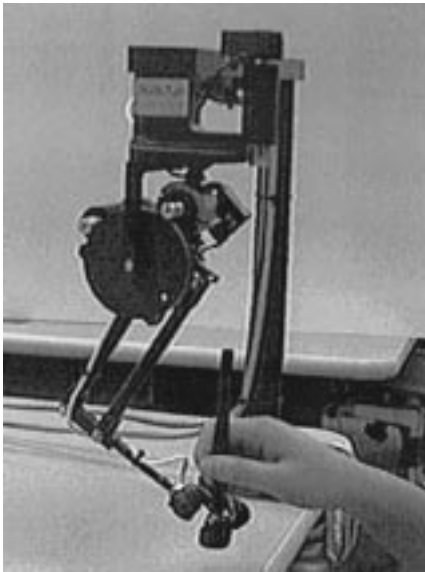
Fig. 3. The PHANToM, as used by the operator for skill demonstration.
