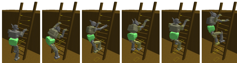
Fig. 10. A ladder climbing primitive adapted to a new ladder with uneven rungs.
