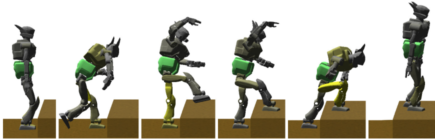
Fig. 4. Stair step planned entirely from scratch.
