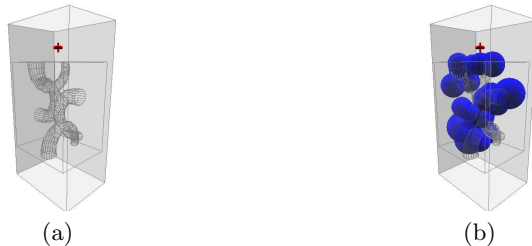
Fig. 7. (a) Maze environment. The robot must pass through a series of passages from the start to the goal configuration. (b) Narrow local regions of C-Space found.
